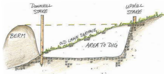
Figure 2. Where to dig and how to create the berm on a sloped site.
